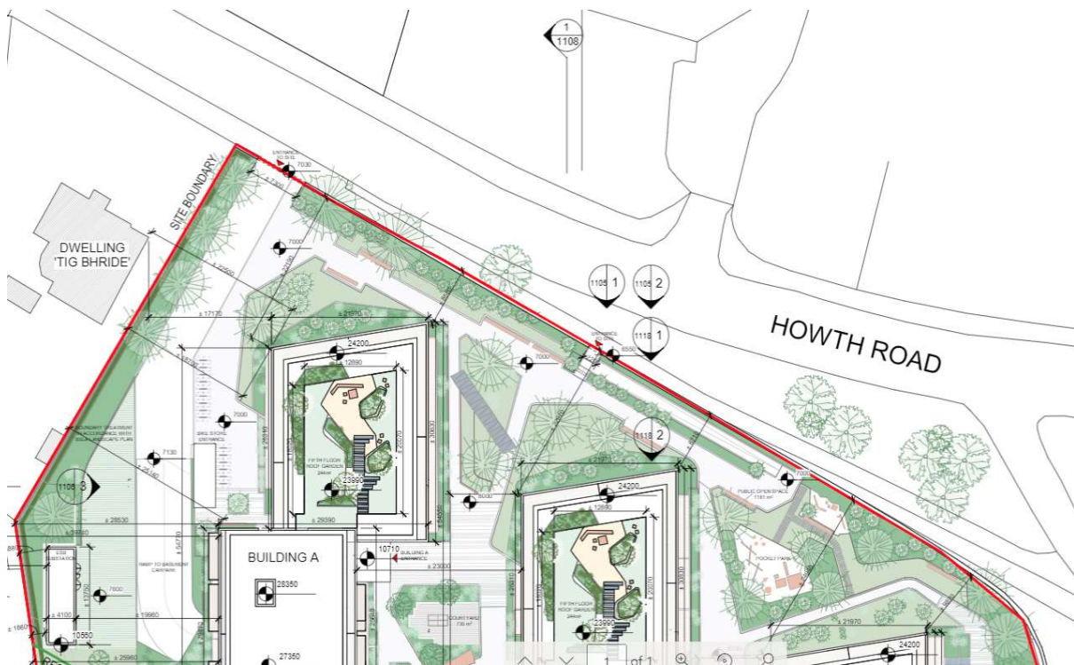
Figure 15.2: Extract from the Proposed Site Layout Plan, showing the location of the two proposed new entrances in the existing boundary wall.
