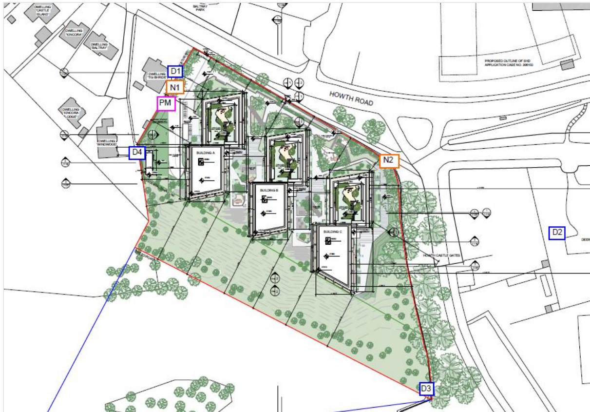
Figure 13.2 Construction Phase Dust (D) Particulate Matter (PM) and Nitrogen Dioxide (N) Monitoring Locations
