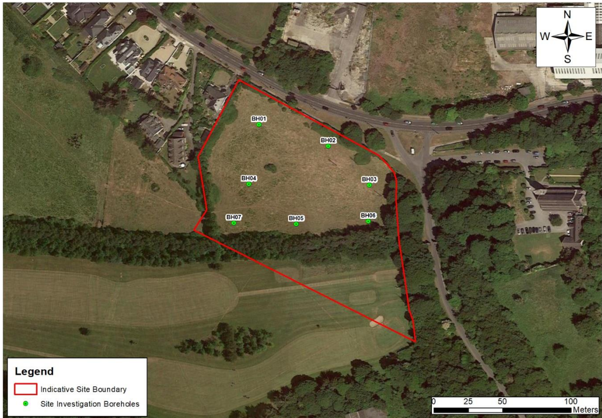
Figure 9.5 Site Investigations Boreholes (Source: SIL, 2019)
